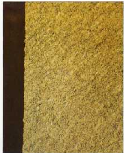
Dezincification Resistant Brass (CZ 132) after testing. At a magnification of x 50 there is no evidence of attack. (Delta Extruded Metals Ltd.)
