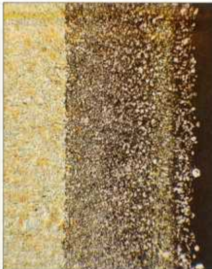
Conventional brass (CZ 122) after exposure to the dezincification test. The photograph (x 50) shows the considerable depth of dezincification attack with extensive porosity to a depth of 1 mm from the surface. (Delta Extruded Metals Ltd.)
