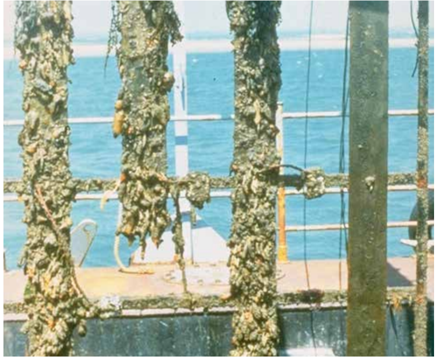
Exposure panels (left to right in above picture): steel, 90-10 copper-nickel sheathed steel, copper-nickel - all three protected with aluminium anodes - and freely exposed copper-nickel. After 12 months exposure at Langstone Harbour, UK, there was no macrofouling on the freely exposed panel.
