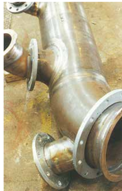
90-10 copper-nickel pipe fabrication for ship seawater system
