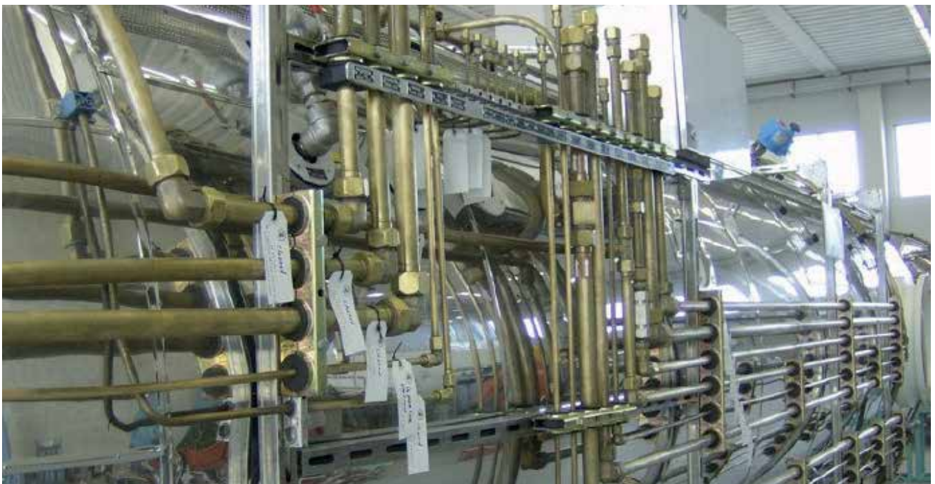
Figure 7 - Tungum® brass tubing on decompression chamber housing living and sleeping sections for divers (Courtesy Drass Galleazzi Underwater Technology)
