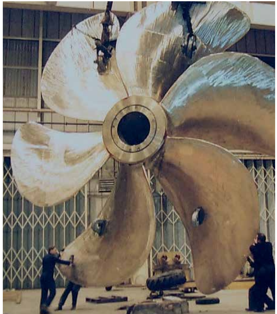
Figure 4 - Nickel aluminium bronze ship propeller (Courtesy Stone Marine Propulsion)
