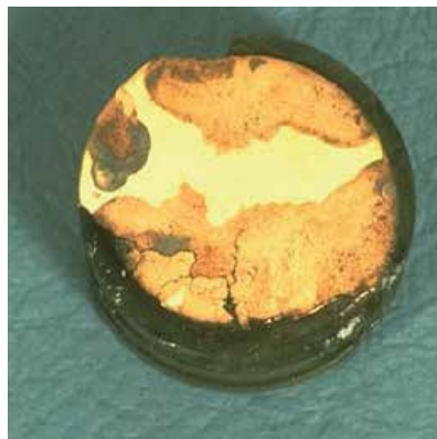
Figure 9 – Dezincification of a 60-40 brass valve stem
