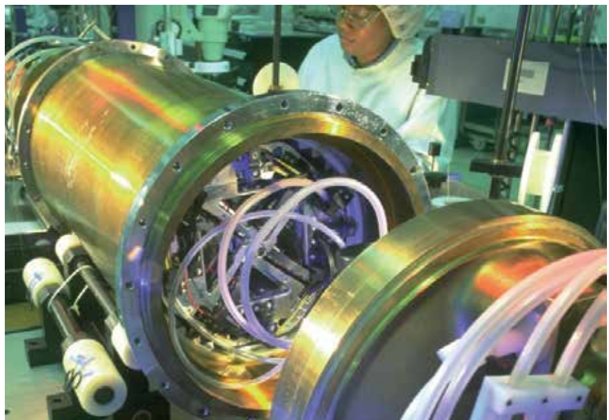
Figure 8 – Copper-beryllium repeater housing assembly (Courtesy Materion Brush Performance Alloys Ltd)
