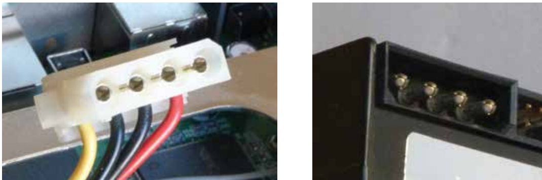
Figure 10 – Connectors using pin and sleeve contacts
