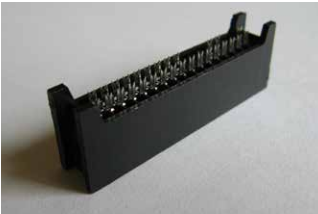
Figure 18 – The cable interface of an IDC connector
