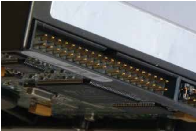
Figure 16 – A PCB header for use with an IDC header of the type shown in Figure 15
