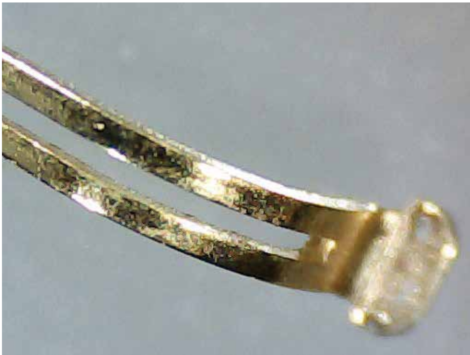
Figure 14 – The gold plated contact surface at about 40x magnification
