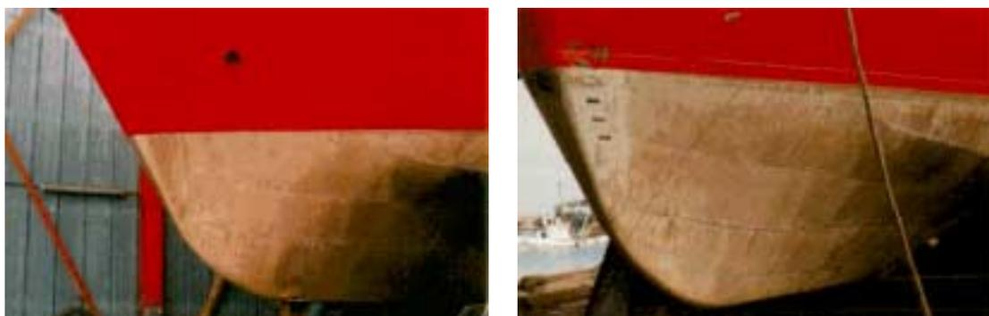
*Figure 11 - Hard shell fouling on the coal tar epoxy coated propeller shaft tunnel after 2.5 months in service*
