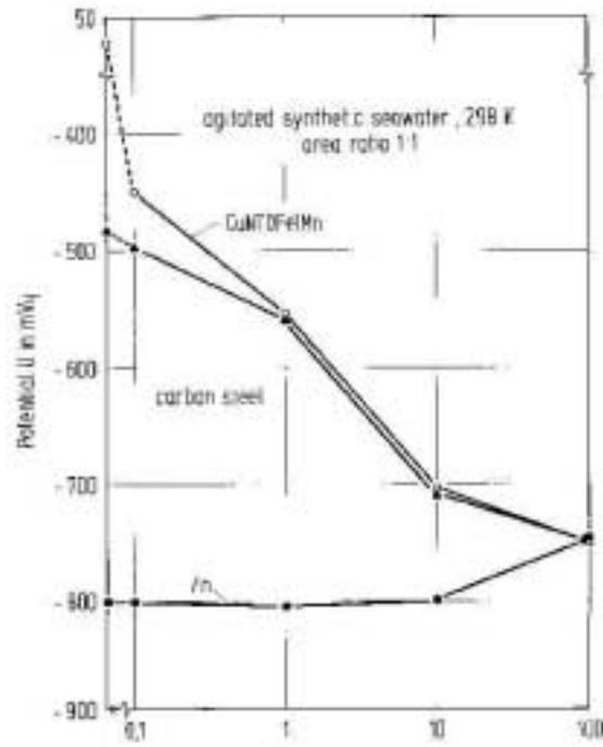
Figure 3 – Corrosion potential of CuNi10Fe1Mn temporarily coupled with a zinc anode
