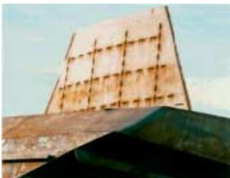
*Figure 8 - Boat stabilizing rudder sheathed on one side with 3 mm CuNi10Fe1Mn-sheet*
