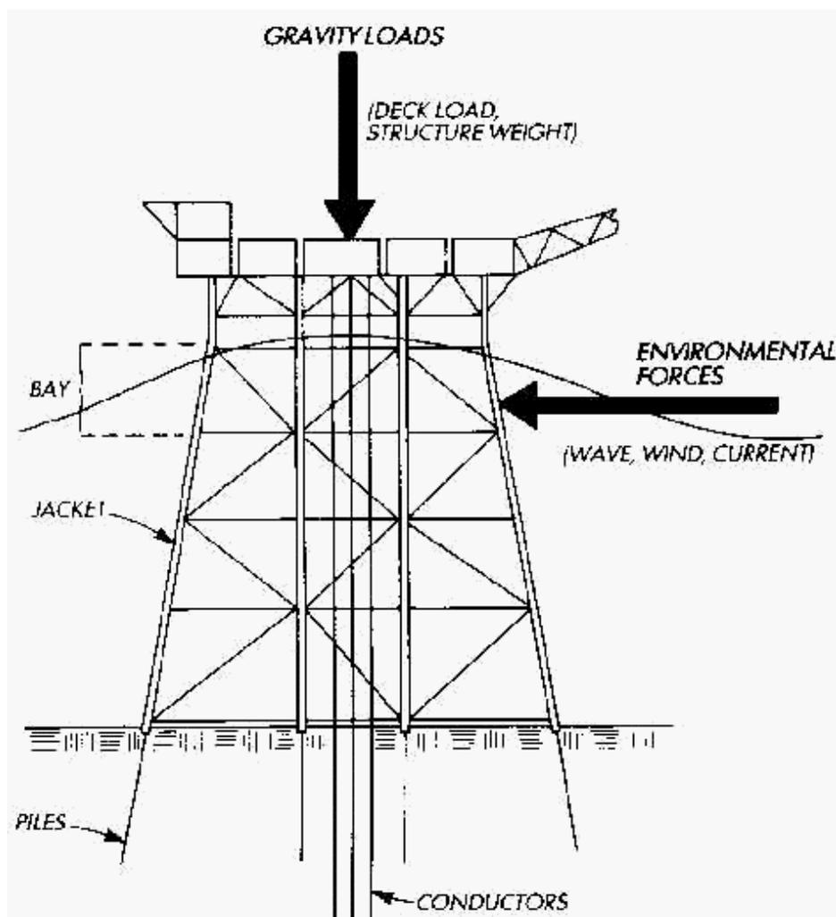
The investigation examined platforms in three water depths for environmental conditions ranging from mild to severe and for marine growth ranging from light to heavy. Using computer-aided design techniques conceptual platform designs were developed to determine the potential savings in jacket and pile steel that would result from the use of copper-nickel sheathings. (Figure 2).
