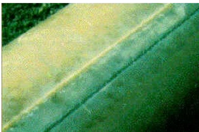
*Close-up of copper-nickel alloy cladding - overlapped and welded joint
