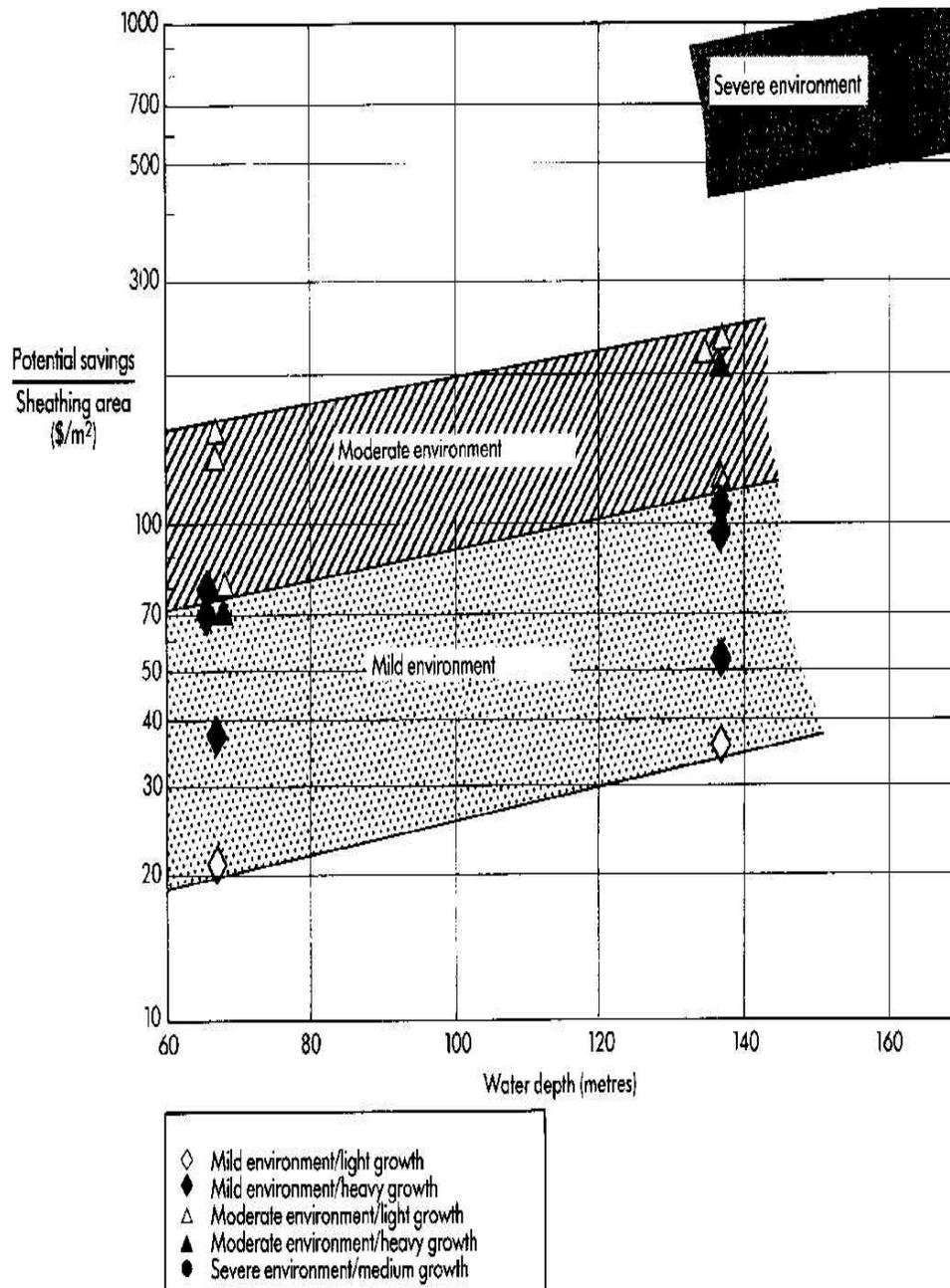
In severe weather environments like the North Sea (design wave height of 90 ft), copper-nickel sheathing would reduce the total platform and pile cost by about 9%, corresponding to roughly \$8.7 million in potential savings in material and fabrication cost. In moderate environments, typical of the Gulf of Mexico (design wave height of 71 ft), the weight savings for the extreme case amounted to about \$0.9m, or about 6% of the total platform cost. Even mild environments,
