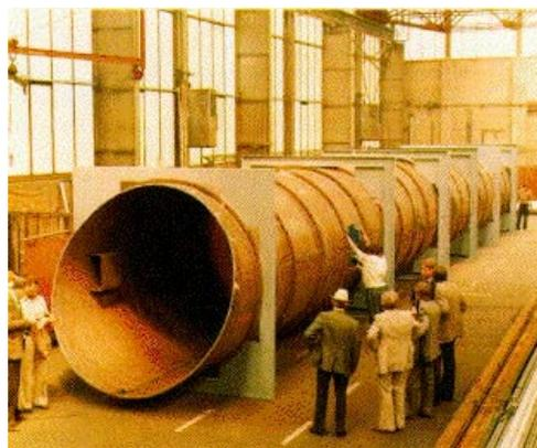
Figure 5 - Seawater suction pipe for the fire extinguishing plant at Jeddah airport in Saudi Arabia.(photo: VDM).
