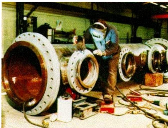
*Figure 4 - 90/10 Copper-Nickel inlet/outlet manifolds for Seawater Course filtration unit
