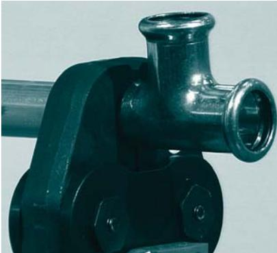
force is always used to create a sound joint. A safety clutch switches the machine off as soon as maximum pressing force is attained. The tool is easy to use. Some tools also have additional features, such as an automatic monitoring function to ensure consistent jointing quality.
