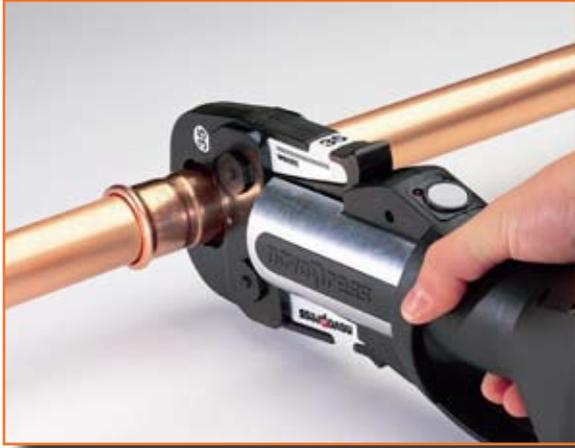
With changes in working practices and construction techniques, there is a demand for faster, cleaner, safer pipework installation practices. Advances in technology have led the copper industry to develop jointing techniques that complement the tried and trusted capillary soldering and compression fittings. The introduction of copper push-fit and press fittings has given installers more jointing options, providing a flame-free solution to meet modern construction techniques.
