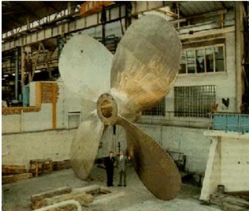
*Weld-repairs can be carried out on castings as large as this 80-ton propeller.*
