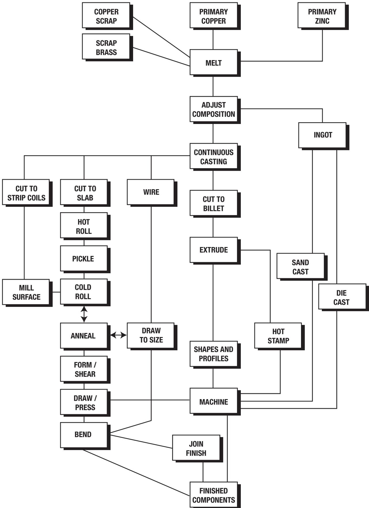
The strength of most of the commercially available brasses cannot be improved by heat treatment. Any improvement in properties over the soft, annealed condition is obtained by cold working. In the case of extruded products such as rods, bars, sections, tubes and wire, the cold reduction is applied by drawing through dies, while in the case of sheet and strip it is applied by cold rolling.
