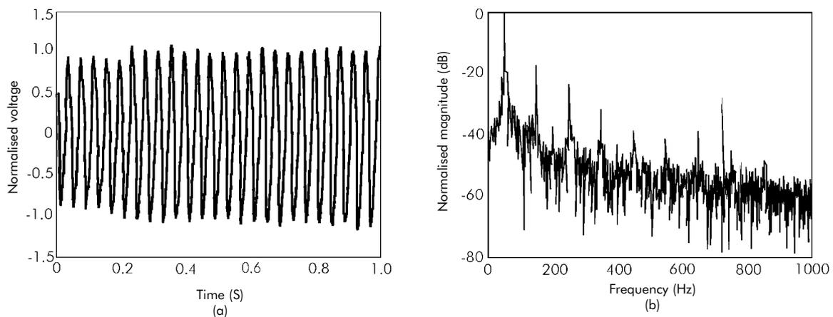
Figure 1 - Typical arc furnace voltage flicker measured at the supply transformer secondary
