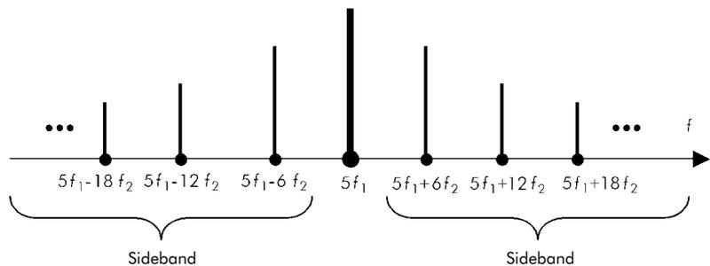
Figure 4 - Sidebands adjacent to the characteristic 5<sup>th</sup> harmonic of a six-pulse converter  $P1$  and  $P2$
