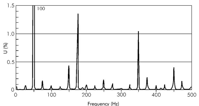
Figure 10 - FFT results for the voltage during emission of data transmission signal ( $U_{ih} = 1.35\%$ ,  $f(U_{ih}) = 175$  Hz)
