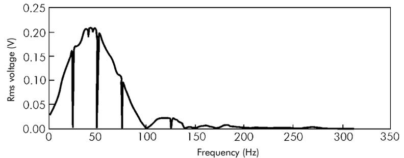
Figure 12 - Dependence of maximum rms voltage variation on the frequency of interharmonic of a constant amplitude (0.2% of the fundamental component amplitude)[10]
