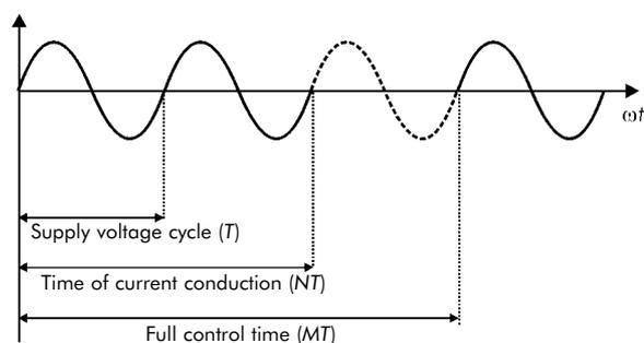
Figure 8 - Waveform of a load current in the integral cycle controlled system:  $N = 2$ ,  $M = 3$
