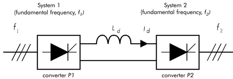
Figure 3 - Indirect frequency converter with a load commutated inverter
