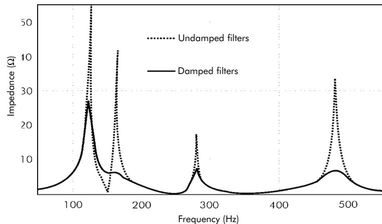
Figure 17 - Example of impedance seen from converters' terminals [10]
