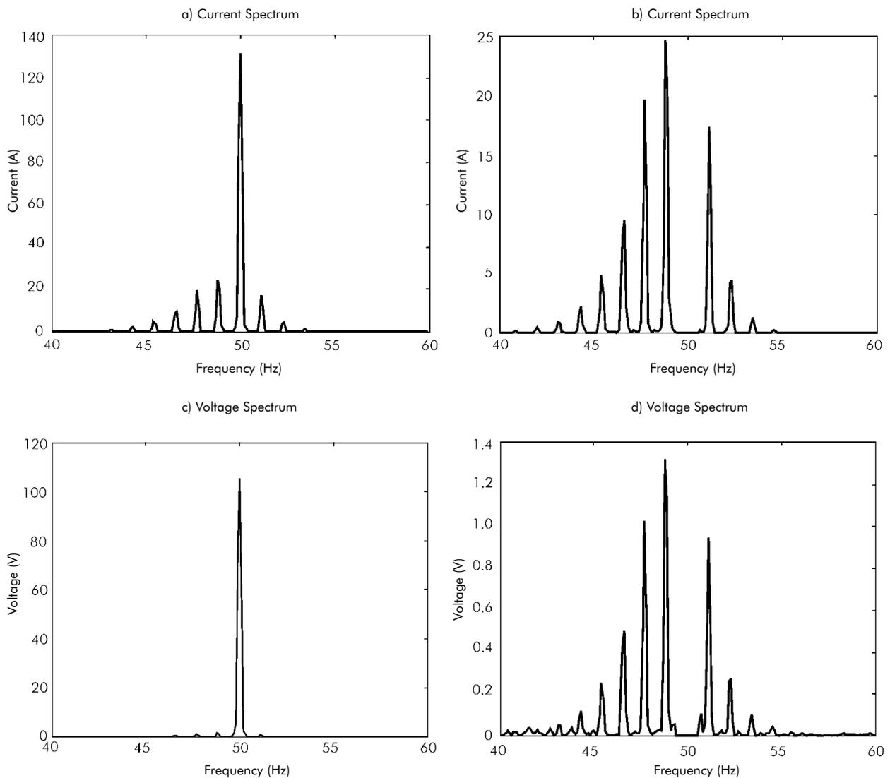
*Figure 2 - Results of the spectral analysis of the motor phase current and voltage at the motor terminals*
