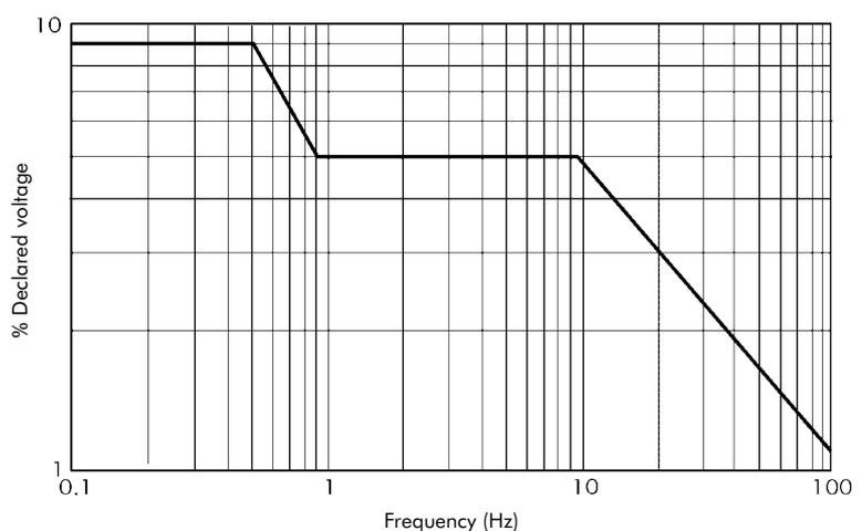
Figure 16 - Voltage levels of signals used in public MV distribution systems [11]
