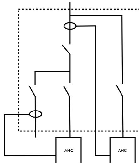
Figure 7 - Cascade configuration
