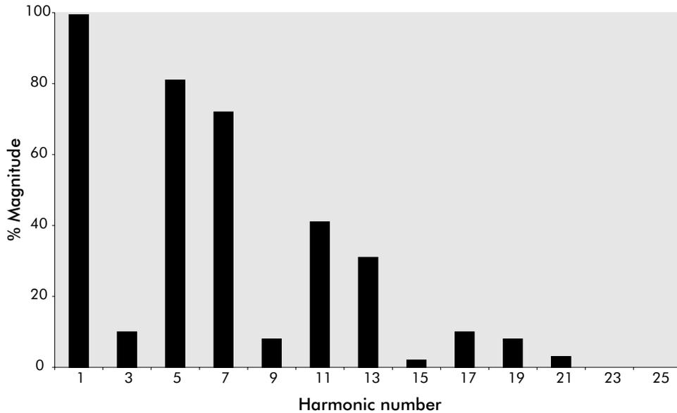
Figure 11 - Typical uncorrected variable speed drive load
