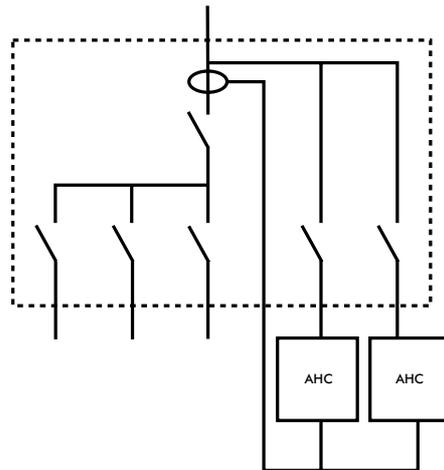
Figure 6 - Parallel configuration
