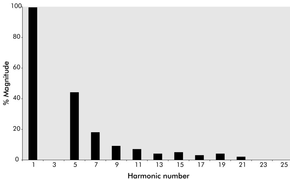
Figure 10 - Partially corrected PC type load
