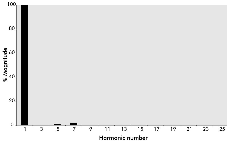
Figure 9 - Completely corrected PC type load
