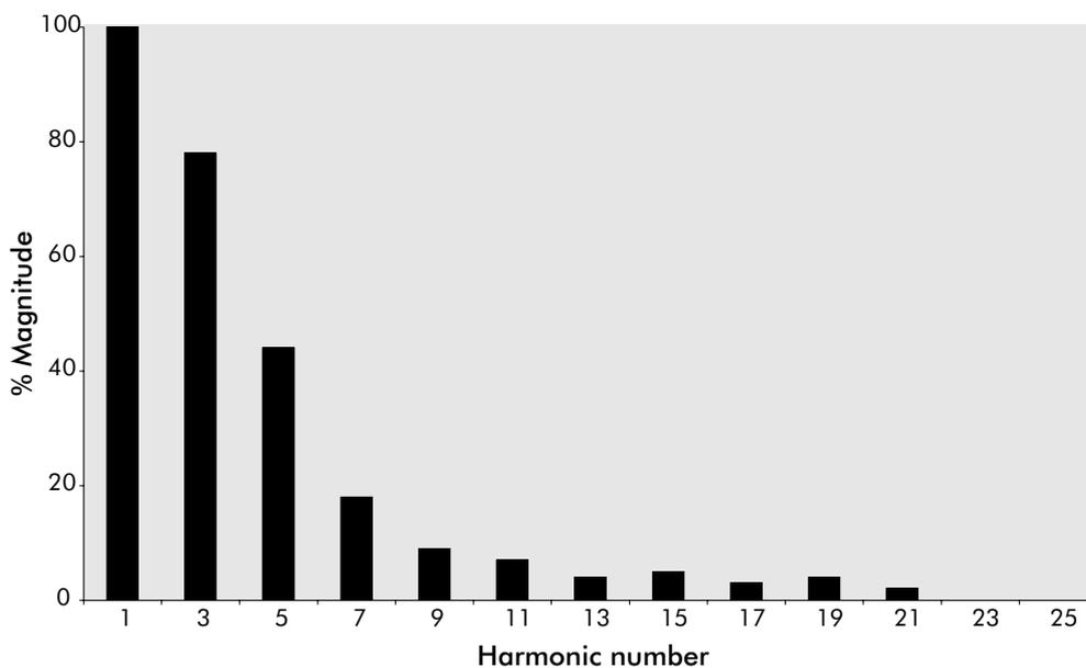
Figure 8 - Uncorrected profile of PC type loads
