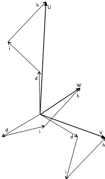
Figure 2 - Graphical decomposition using the components in Figure 1 (the respective contributions to the three phases as indicated with U, V, W are added as phasors to obtain the actual unbalanced system)
