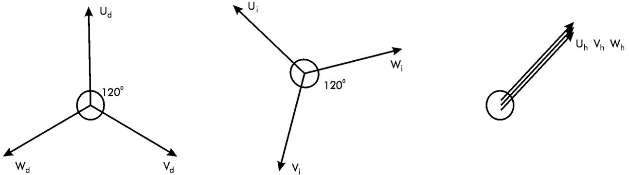
Figure 1 - Graphical representation of the symmetrical components; note the inverse labelling of the positive sequence (leftmost) and negative sequence (middle) contributions to the actual voltage phasors
