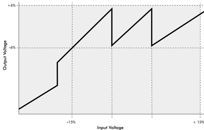
Figure 10 – Input/output characteristics for a step regulator
