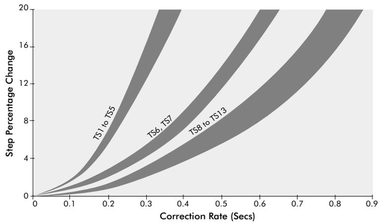
Figure 5 – Typical correction ratios against step percentage change - Type 80 servo amplifier
