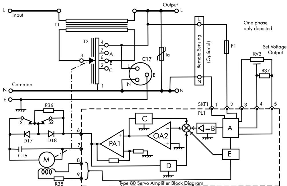
Figure 1 – Basic circuit diagram of electro-mechanical voltage regulator
