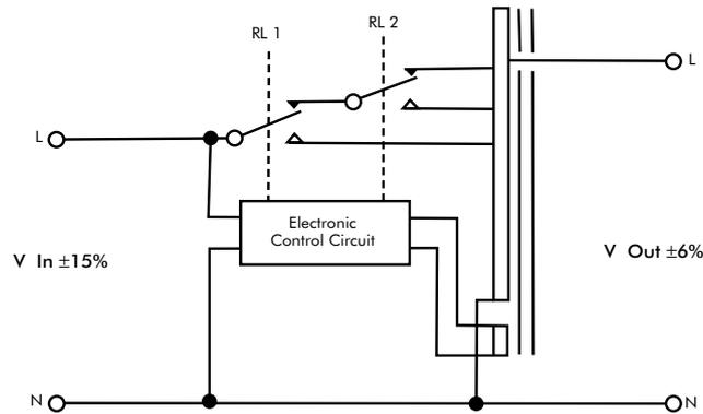
Figure 9 - Basic circuit of a step regulator
