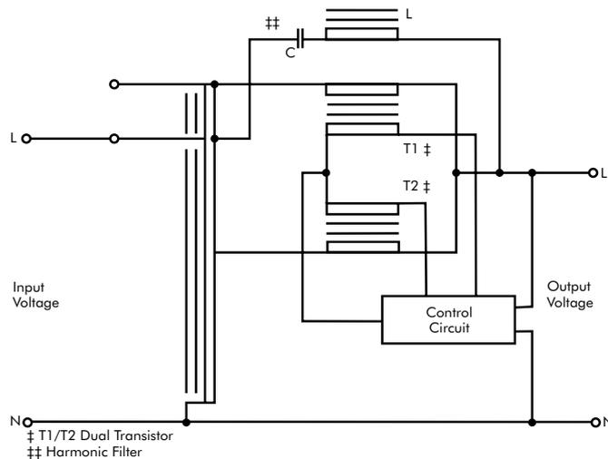
Figure 11 – Circuit of a saturable reactor regulator
