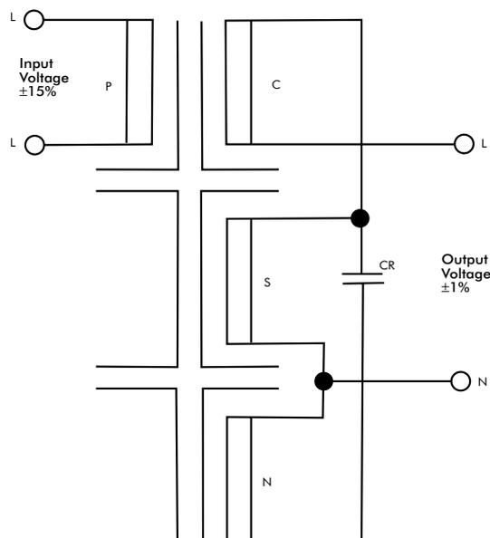
Figure 7 – Basic circuit of CVT
