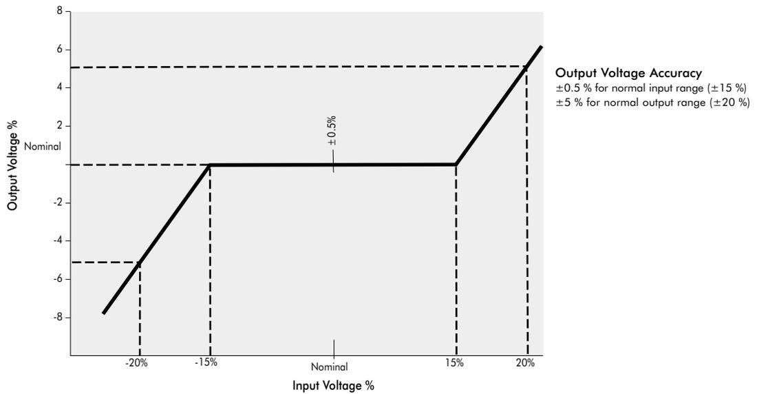
Figure 2 – Input/output characteristics for a  $\pm 15\%$  stabiliser
