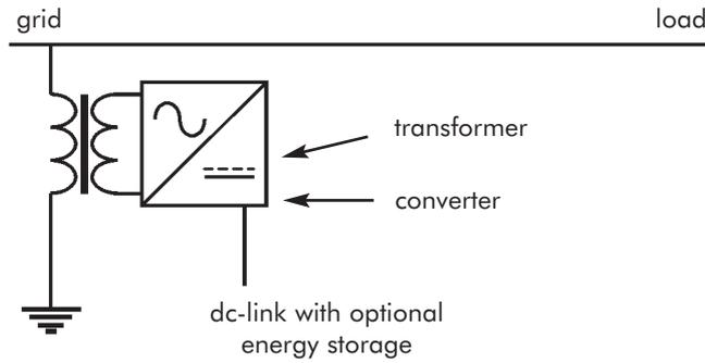
Figure 6 - Block diagram of a statcom
