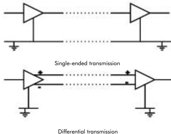
Figure 4 - Single ended (top) and differential signal interfaces
