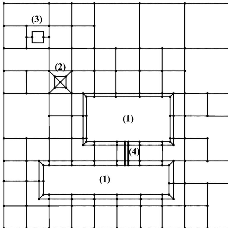
Figure 2 - Earth grid (after Figure 8 of IEC 61312-2)
