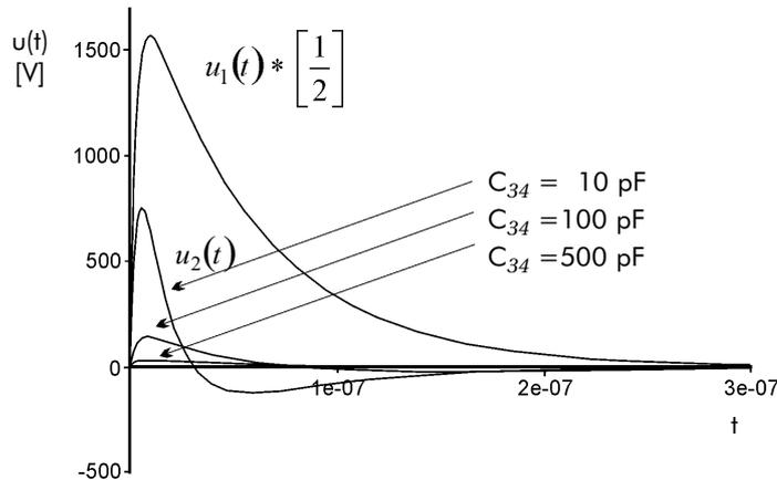
Figure 16 - Shielding of a burst pulse by shields of a different internal capacitive coupling
