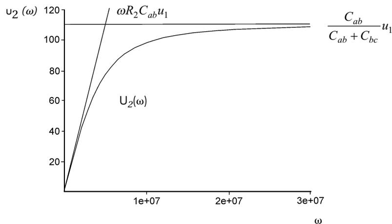
Figure 13 - Frequency behaviour of the capacitive coupling
