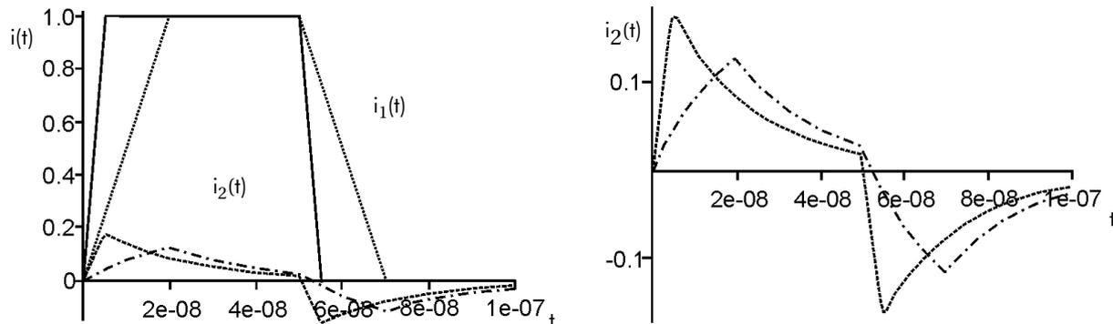
Figure 9 - Inductive coupling of slow and fast trapezoidal currents
