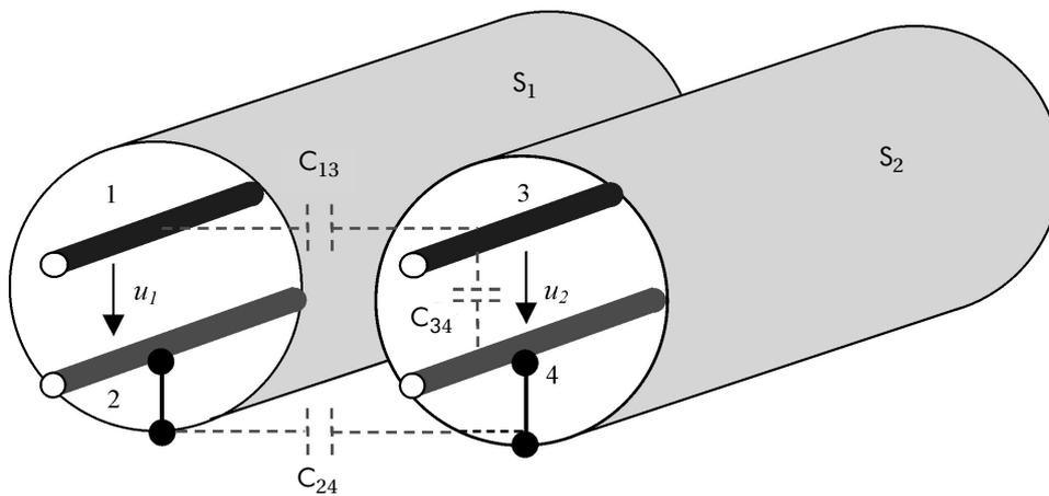
Figure 15 - Capacitive coupling of two shielded cables
