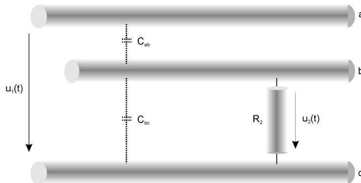
Figure 12 - Three line model for capacitive coupling
