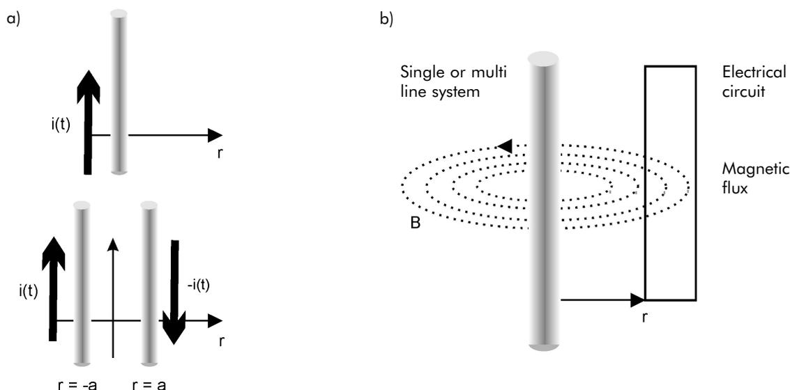
Figure 5 - a) A single and a go-and-return line as sources of a magnetic field
