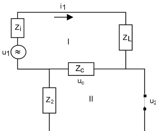
Figure 2 - Impedance coupling
