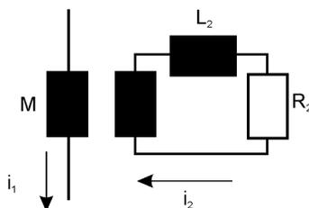
Figure 7 - Equivalent circuit for the inductive coupling
