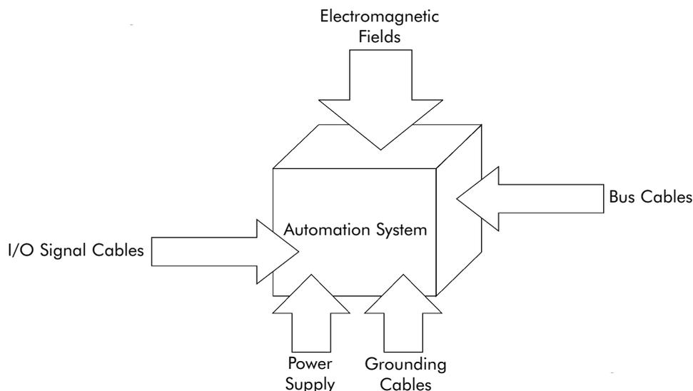
Figure 18 - Various couplings paths of an automation system
