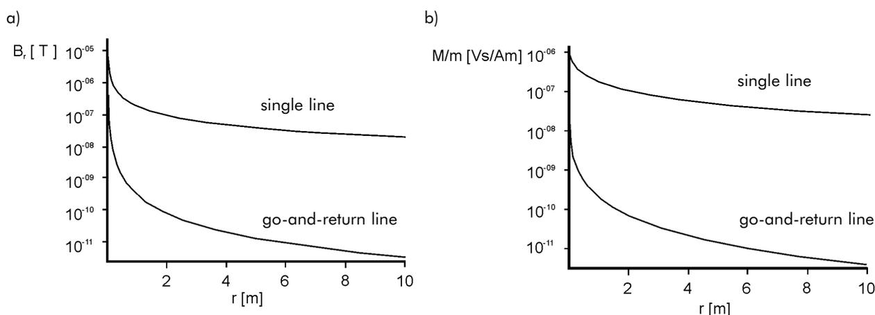
Figure 6 - a) the magnetic field of a single and a go-and-return line
