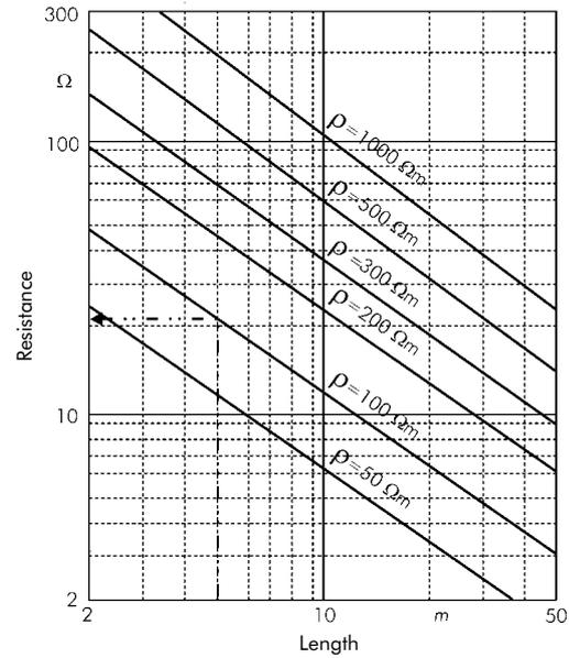
Figure 5 - Earth resistance (dissipation resistance) of a rod electrode with length  $l$  and diameter  $0.02$  m in a homogenous ground with resistivity  $\rho$  [2]
