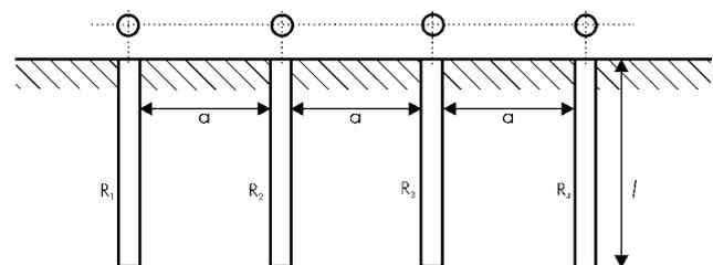
Figure 6 - Parallel placed rod electrodes;  $R_1 - R_4$  - individual resistances of electrodes,  $a$  - electrode distances,  $l$  - electrode length
