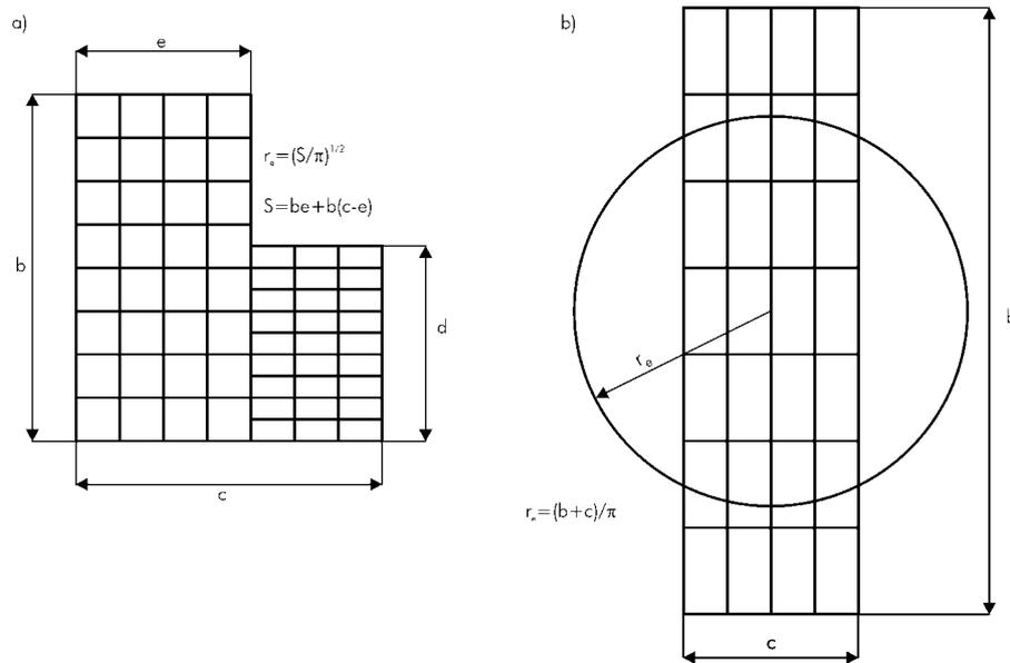
Figure 7 - Examples of meshed earth electrodes explaining the method of calculation of the equivalent radius  $r_e$  in equation (11), for two forms of the earth electrode: nearly similar to a square (a) and a long rectangle (b)
