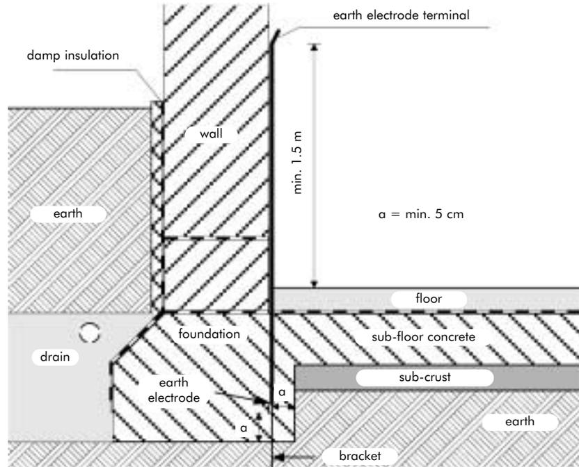
Figure 8 - Illustration of the placement of the foundation earth electrode in a foundation without concrete reinforcement
