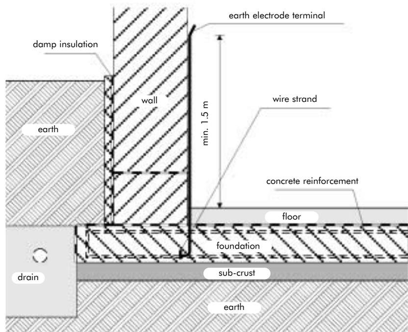
Figure 9 - Illustration of the placement of the foundation earth electrode in a foundation with concrete reinforcement
