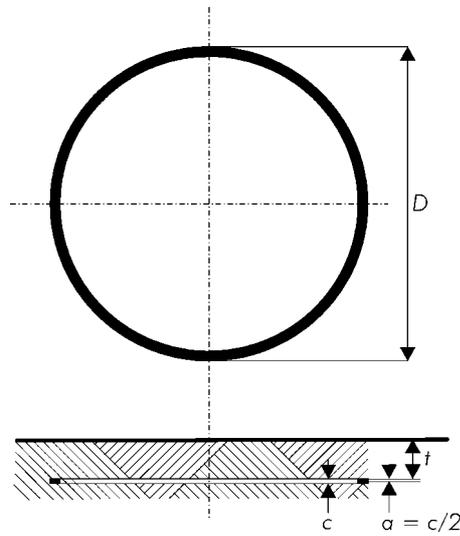
Figure 2 - Diagram of a simple ring earth electrode, according to equation (8)
