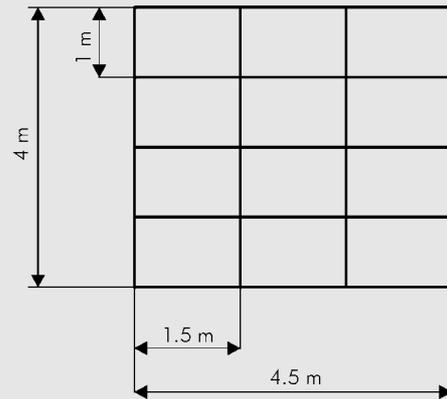
Figure 10 - Sketch diagram of the meshed earth electrode (Example E)
