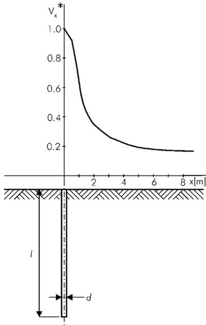
Figure 4 - Earth surface potential distribution  $V_x^* = f(x)$  around a vertical rod earth electrode with length  $l = 3$  m, diameter  $d = 0.04$  m
