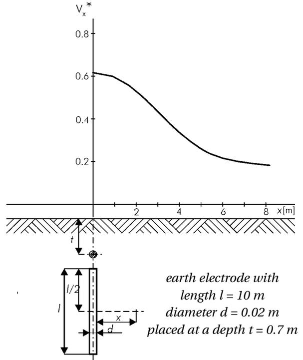
Figure 1 - Earth surface potential distribution perpendicular to the horizontal pipe
