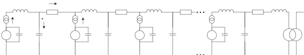
Figure 12 - An example of a wind farm consisting of six turbines arranged in a string
