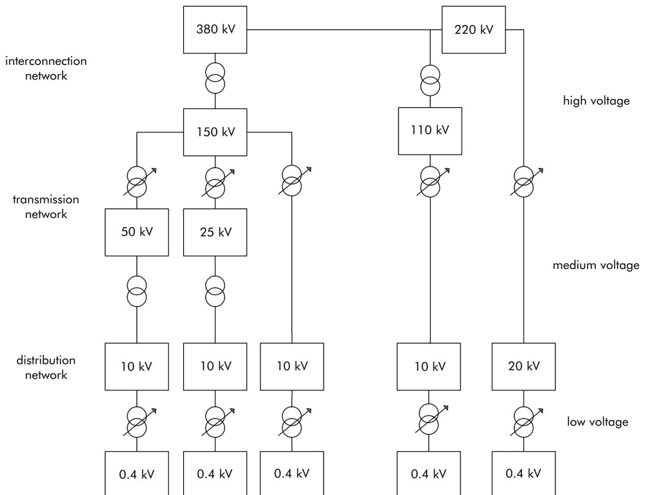
Figure 1 - A typical electricity network with centralised generation on the 380kV transmission network
