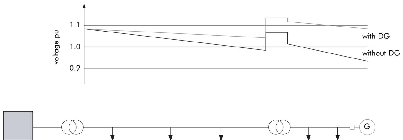
Figure 10 - Voltage rise due to reversed power flow due to DG
