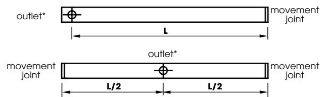
\* Outlets should be detailed to allow free movement between the spigot and substrate of 5mm in each direction
