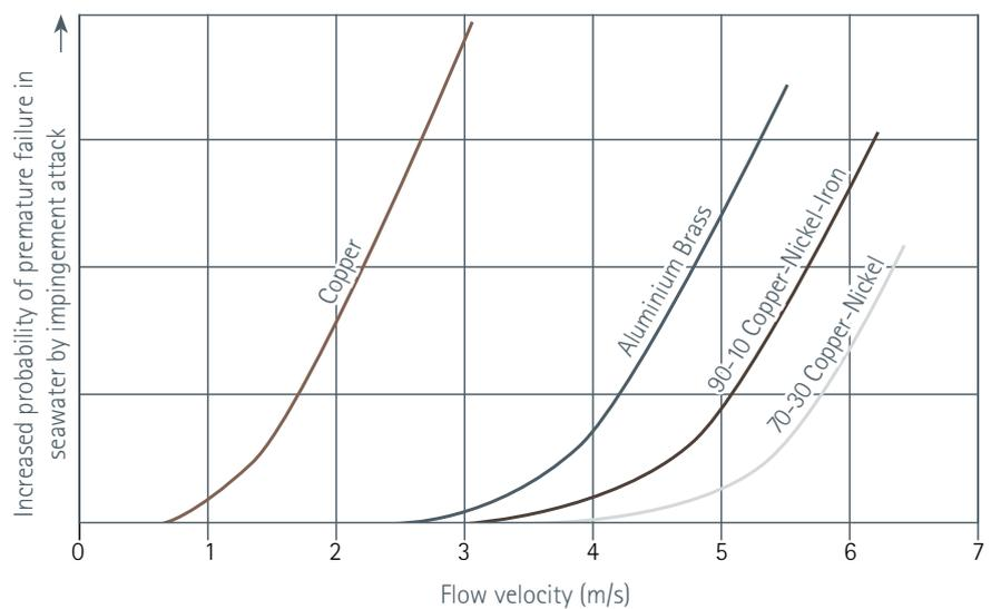
Figure 11 - Relative breakdown velocities for copper alloys in seawater ex Gilbert<sup>(22)</sup>
