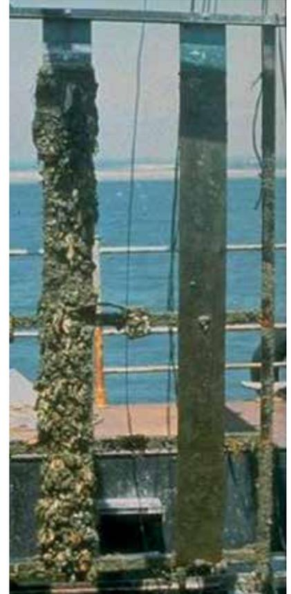
Figure 15 - Comparison of a cathodically protected (left) and freely exposed 90-10 copper-nickel panel (right) after 12 month exposure at Langstone Harbour, UK. The panel free of cathodic protection remains clean, apart from biofilms (no macro-organism attachment).<sup>(29)</sup>
