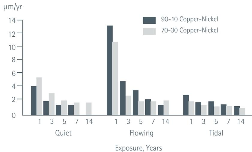
Figure 3 – Fourteen year corrosion rate data<sup>(2)</sup> at LaQue Center for Corrosion Technology, North Carolina, for 90–10 and 70–30 copper-nickels
