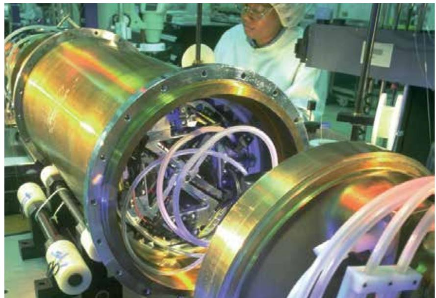
Figure 8 – Copper-beryllium repeater housing assembly (Courtesy Materion Brush Performance Alloys Ltd)
