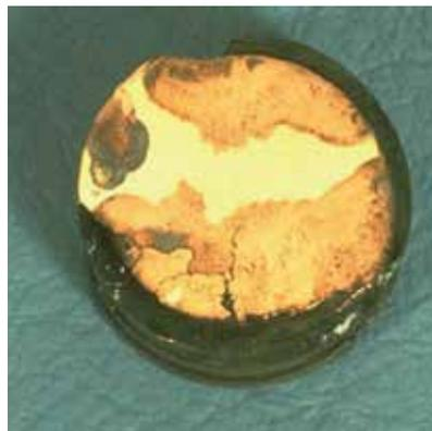
Figure 9 - Dezincification of a 60-40 brass valve stem
